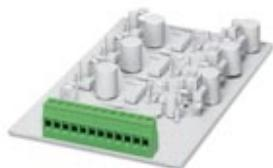
PCB terminal block, nominal current: 24 A, rated voltage (III/2): 400 V, pitch: 5.08 mm, number of positions: 4, connection method: Screw connection with tension sleeve, mounting: Wave soldering, conductor/PCB connection direction: 0 °, color: green, Solder pin [P]: 3.7 mm
